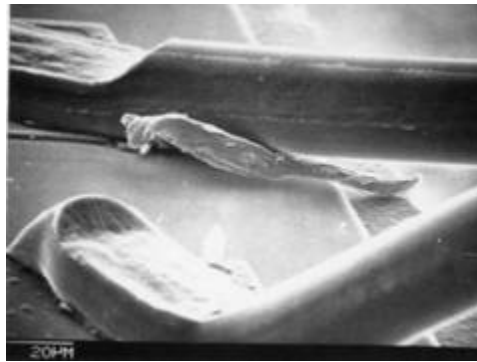
A small metal flake as shown above can cause serious malfunction in electronic components
